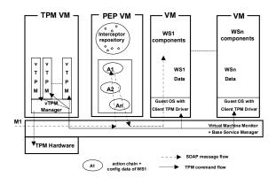
Figure 6: Proposed "TCP-PEP" partition architecture for WS instances
