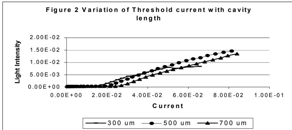
The characterisation of the laser made from the P-PAID sample was done using the conditions given in the previous section and is compare to that of as-grown laser. The variation of threshold current with cavity length as predicted by theory is shown in Figure 2. Table 1 gives the parametric values obtained.
