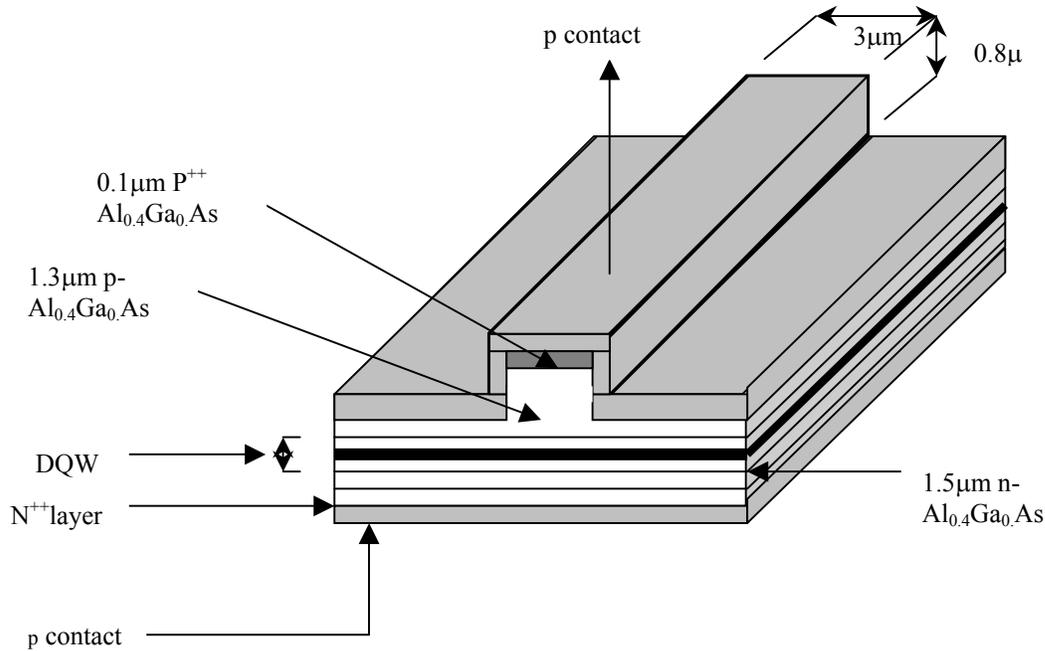
Figure 1 : Ridge waveguide double quantum well GaAs/AlGaAs laser
